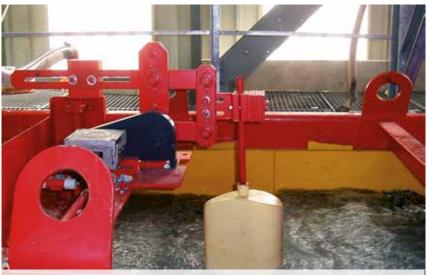
View of the water box and the automatic float switch
