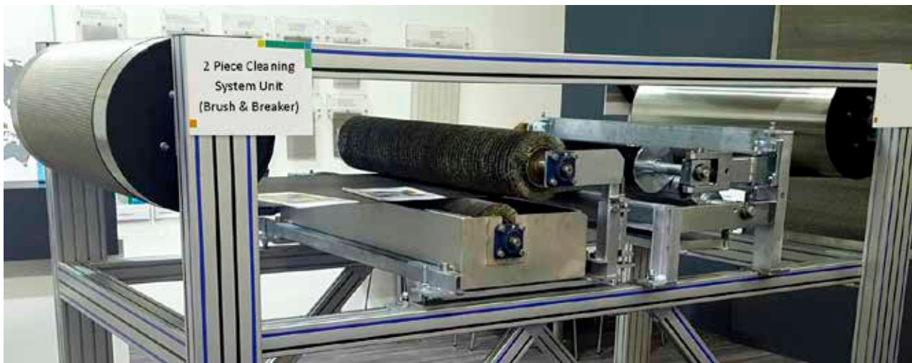
Exhibit model of a belt cleaning system unit consisting of "dirt breaker" & "dirt swiper"
