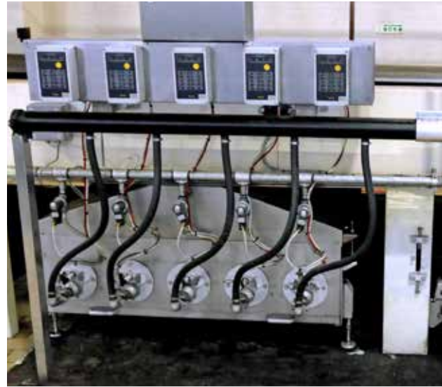
This is a dirt burning station at oven's exit, which did not work successfully and was consequently switched off.
