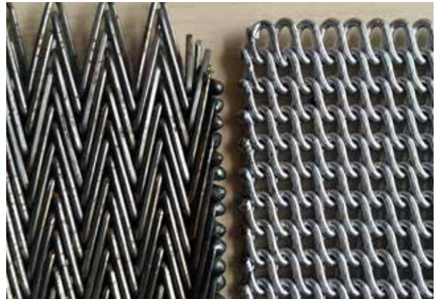
Balance weaved CB5 (left) replaced by Z-Belt F4018 (right)
