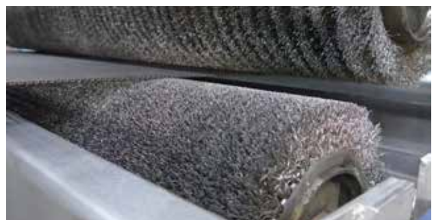
These pictures show essentials of a good brush system: upper & lower brush of different design
