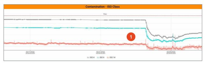
After starting the bypass flow filtration (1), solid contamination is significantly reduced.
